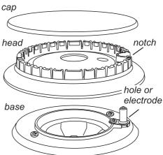
When refitting the burner head, make sure that the notch lines up with the electrode or hole in the base. Check that the burner head is level and that the cap is fitted centrally on the burner head.
